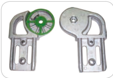
Aluminium die casting hinge with polyamide clutch insert to avoid the material wear and tear
